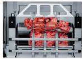
Model型號 Fromat 053 Cutting area切件尺寸: 480x250mm Product temperature被切件溫度: -25 degree C Dimension尺寸937x2666x1920 WxDxH(mm) Electricals電源 400/3/50, 5.5kW
